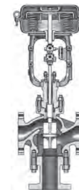
Three way control valve
