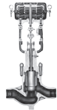
Top guided high pressure single seated control valve
